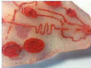
Test piece of microfluidic in soft silicone filled with paint
